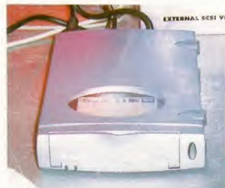
The SyJet from SyQuest not only looks hot, it can also store 1.3Gb on each cartridge.
